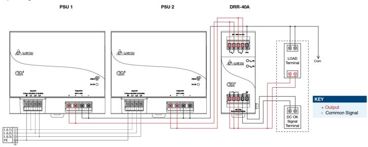
Fig. 3 Redundancy / Parallel Operation Connection Diagram
