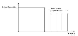
It is not recommended to prolong the duration of  $I_0$  when it is <200% but >100%, since it may cause damage to the PSU.
