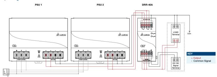
Fig. 3 Redundancy / Parallel Operation Connection Diagram
