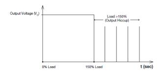
Additionally, if the  $I_O$  is <150% but >100% for a prolong period of time (depending on the load), the Over Temperature Protection (OTP) will be activated due to high temperature on critical components. The power supply will then go into "Hiccup mode" until the fault is removed.
